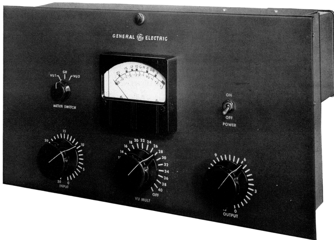
Type BA-7-A Audiomatic Limiting Amplifier
