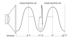
The PHASE switch on the ONBOARD BLENDER in effect electronically "moves" your instrument's position relative to the speaker by inverting the phase 180° every time you flip it.
