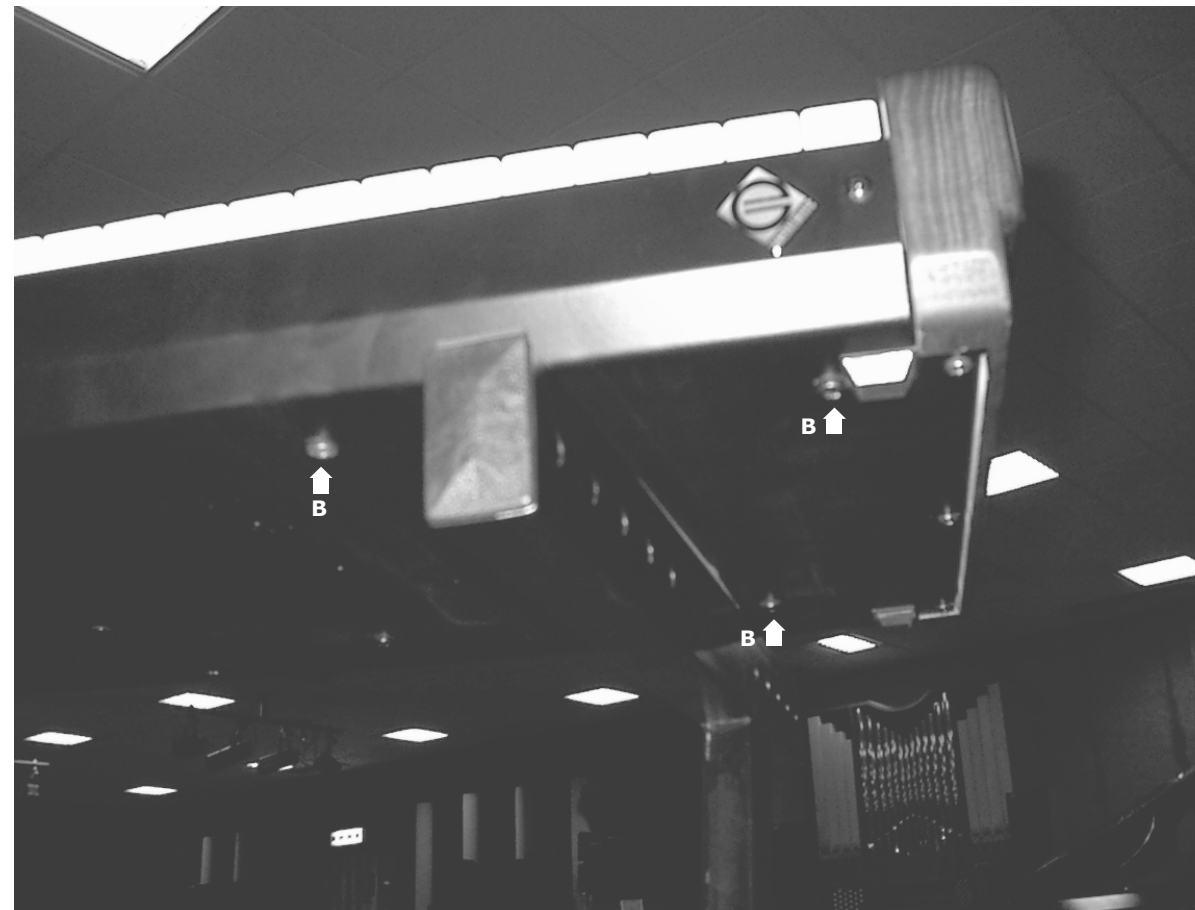
Fig.2 To remove the keyboard unscrew the 11 fixing screws (B) underneath it.
