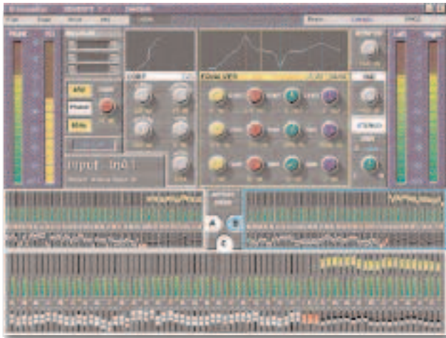
The Sensory display: showing mix, dynamics, EQ and metering information.
