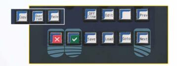
The console is 'frozen' in its current state and the audio continues unchanged. The console software, Sensoft, now lets you change to the page to edit, add this new mic, prepare settings corrections and routing to the buses, and save the new modification. If necessary then OverRam the mic settings to all the pages of the show where this mic is to be used.
