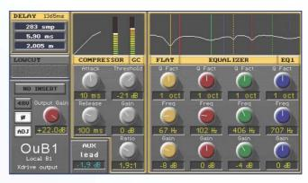
When the outputs are equipped with Hyper-Drive™ audio processing (XO-8D, DO-8X), each output has a complete dynamic processing section - gate and compressor, fully sweepable parametric equalization with eight bands, delay of up to 1.35 second and output level adjustment from +10.5 dBu to +22 dBu. Everything is on-board and immediately accessible. There is no need for external racks, just connect your amplifiers!
