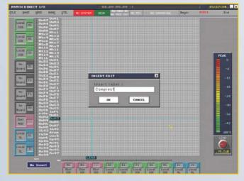
At the heart of the Sy80 console there is a powerful digital audio signal distribution routing and splitting functionality. Accessed by the MUXI key, the I/O page displays this comprehensive switching matrix giving you access for a view of all the system outputs and their assigned processing.
