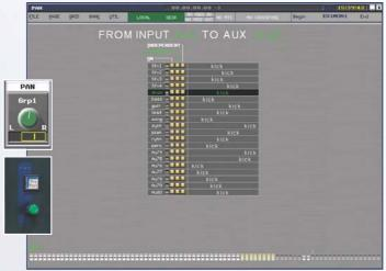
Now press Pre/Post and the full Pan screen opens. By selecting each of your buses, you have control of the corresponding pans and balances immediately, as well as a complete view of the channel panning distribution.
