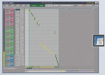
To assign an input to a fader press the Patch IN key in the Patch section, the corresponding screen opens and displays the global assignments to input faders. If you want to add or change an assignment, then select an input fader, choose your physical input (distant or local) with the track ball pointer or keyboard. Right click the trackball button (or hit space bar), and the connection is made.
