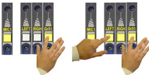
Route Subgroup 51 to one of the Masters
