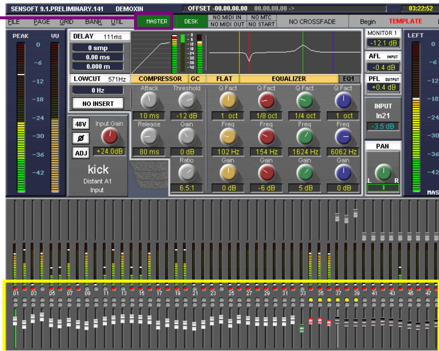
The screen displays the faders in their exact position, their colors reflecting their associated functions.
