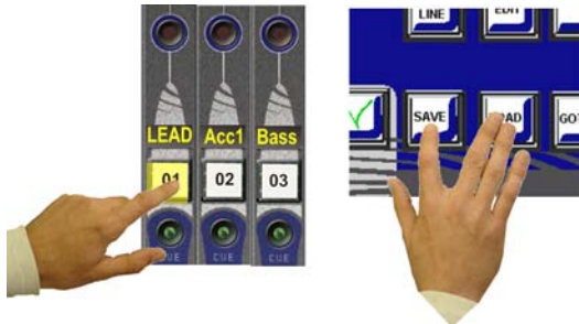
Holding down the [SELECT] button on the relevant channel, and pressing [SAVE] on the console's DESK CONTROL panel is equivalent to selecting Save in the BANK menu
