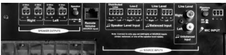
SMS1 INPUT PANEL: The SMS1 System accommodates one music source—such as programmed music, CD player, tuner, or tape player—and one paging microphone. A wide variety of input levels and types are allowed including: balanced line level, speaker level, or unbalanced (RCA) line level.
