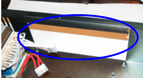
Install power amp (50-00-0163) through this opening
