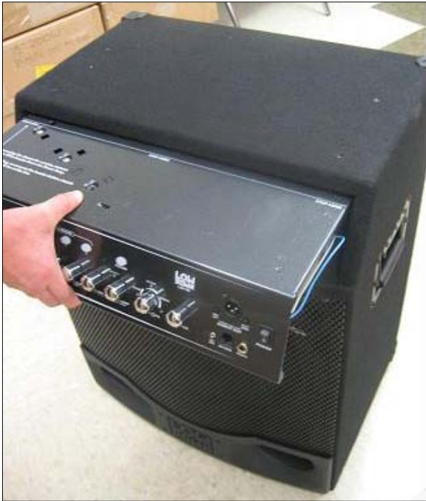
Insert Chassis Assy to Scribe Line
