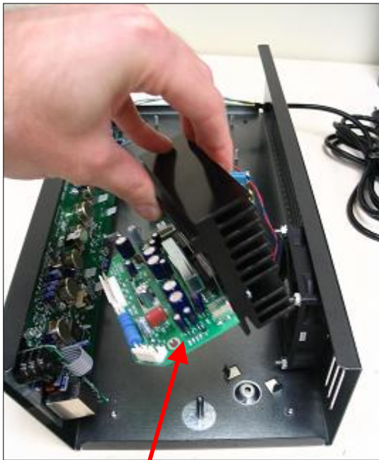
Heatsink/Power Amp PCBA (P/N 50-04-0054)
