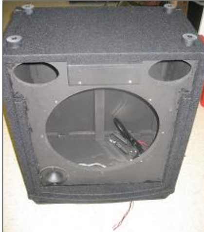
Position the cabinet with the top on the ground
