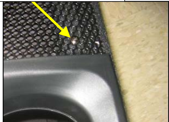
Screw centered on side cleat
