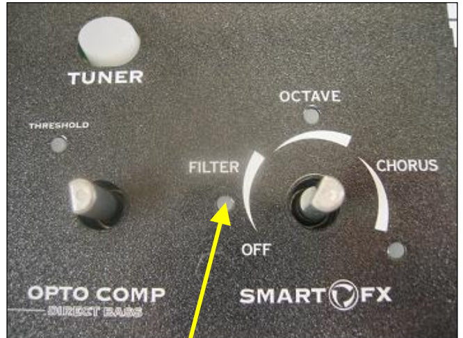
LED cover tips flush with front surface of metal (4 PL)
