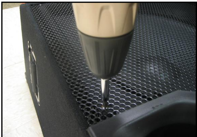
Screw centered on side cleat
