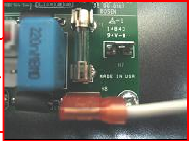
Connect to Header H8
