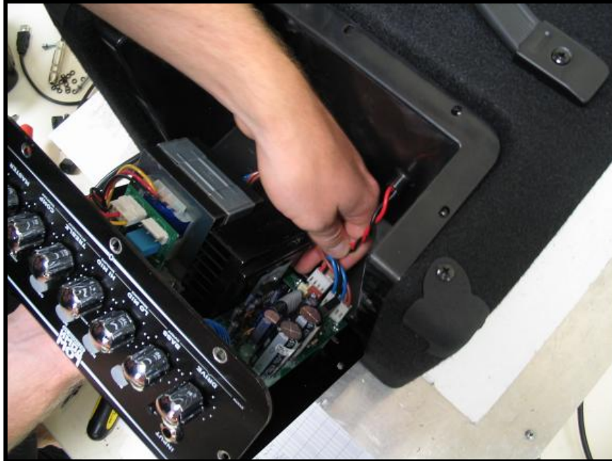
Connect Cable Header to Power Amp
