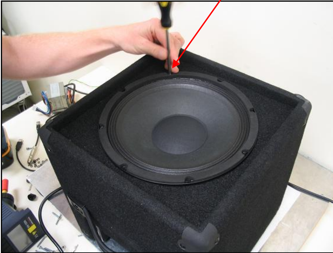
Installation of Speaker Screws
