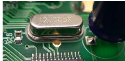
CRYSTAL INSTALLED WITH INSULATOR
