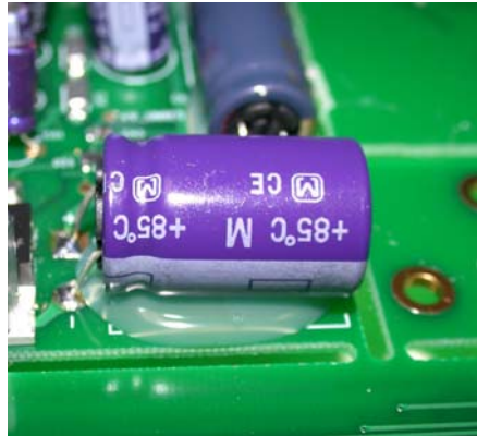
Figure #13: Make sure to add a dab of RTV to C130.
