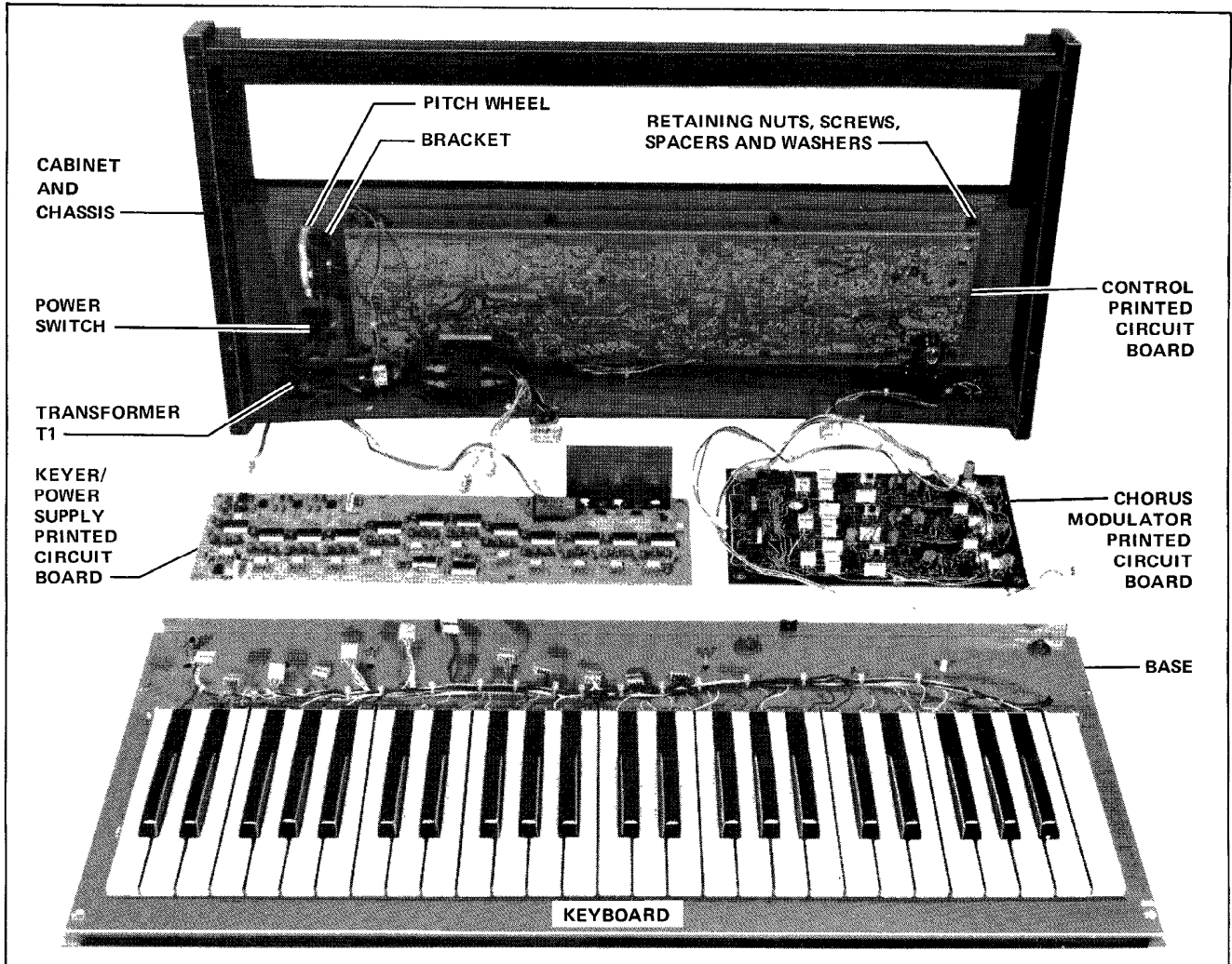
FIGURE 3-2 OPUS 3 WITH BASE REMOVED, KEYSER/POWER SUPPLY AND CHORUS MODULATOR PRINTED CIRCUIT BOARDS REMOVED AND CONTROL PRINTED CIRCUIT BOARD INSTALLED
