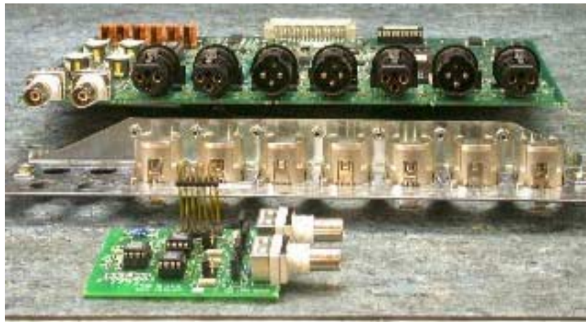
Figure 8: Rear panel removed from FMIO/Composite boards
