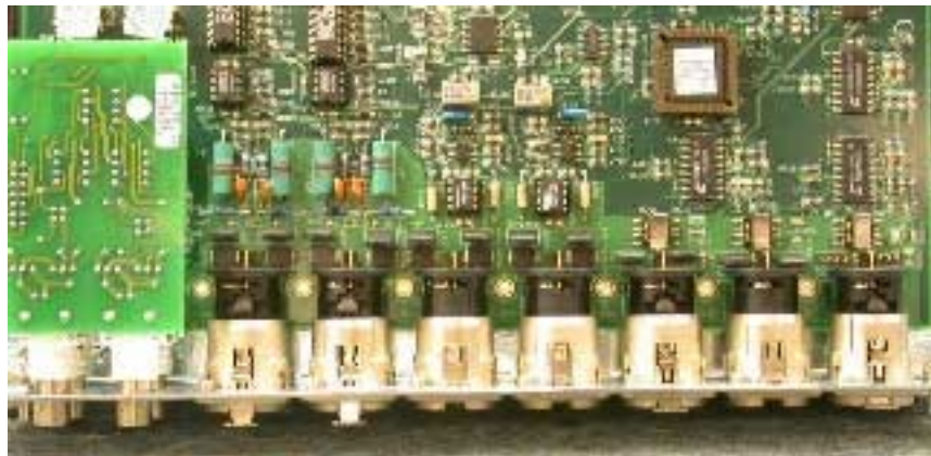
Figure 7: Separating rear panel from circuit boards
