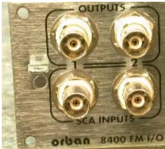
Figure 2: Rear-panel FMIO, BNC detail with hardware
