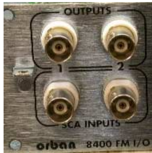
Figure 3: BNC detail, hardware removed
