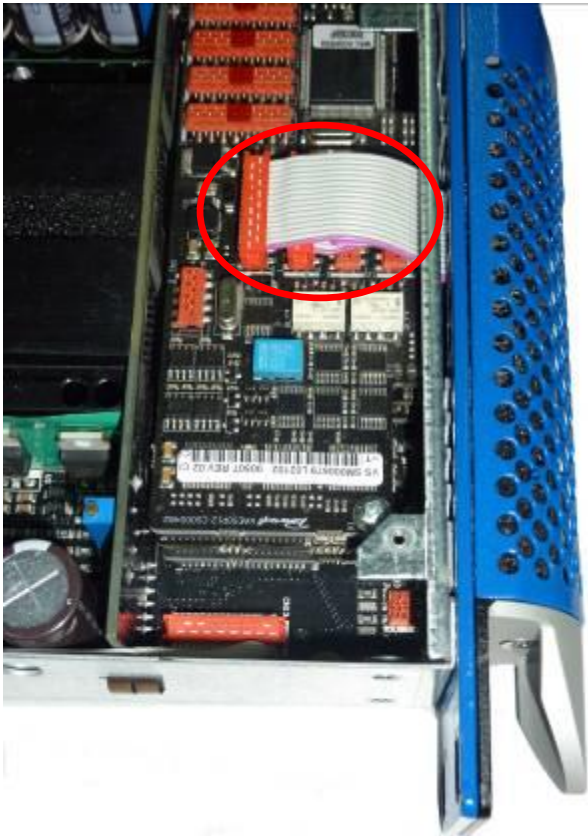
KAESOP flat cable to unplug
