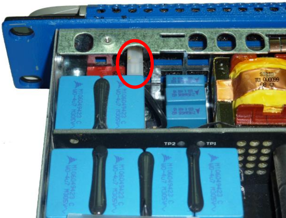
Amplifier power switch cable to be removed
