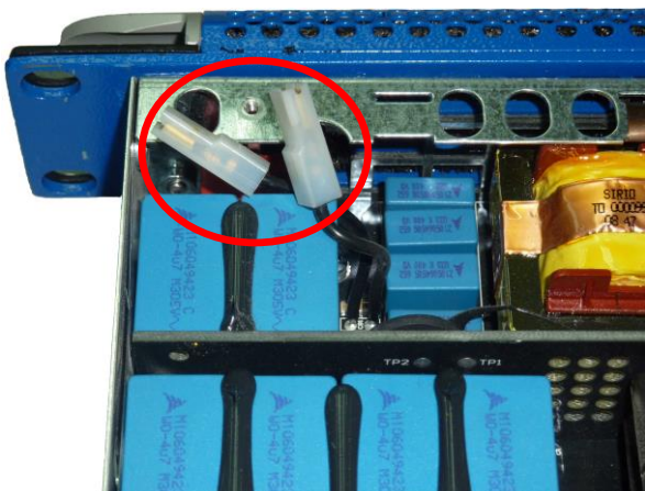
Faston of the amplifier power switch cable removed
