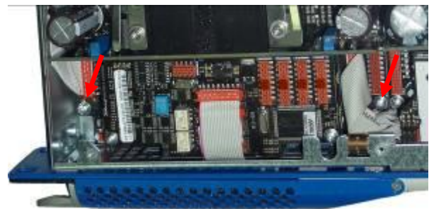
Screw 5 and 6 to be removed
