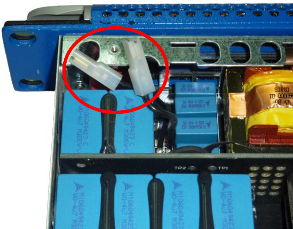
Disconnected faston of the amplifier power switch cable
