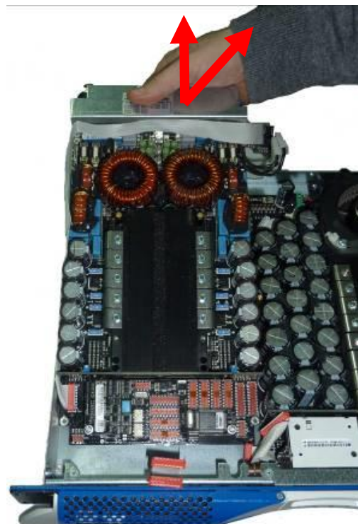
Lift and pull out the amplifier output board from the amplifier chassis
