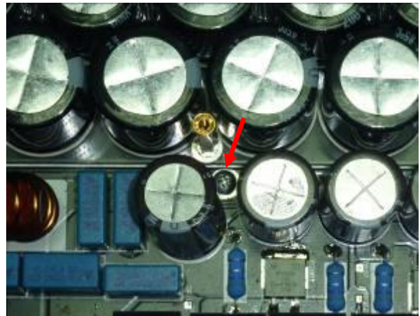
Screw 4 to be removed
