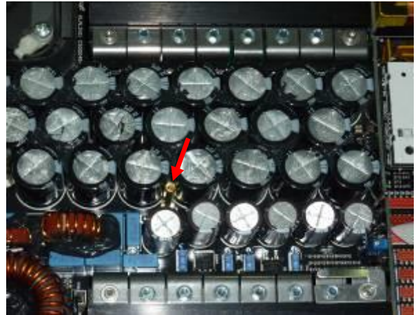
Detail of brass stand-off (screw number 8)
