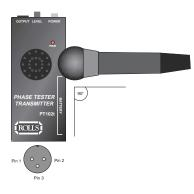
There are a couple of options to check the phase of a microphone. If the mic is dynamic, it may be connected directly to the receiver via an XLR female to 1/4" TS unbalanced male cable. The tip of the 1/4" plug must be wired to pin 2 of the XLR plug, and pin 1 and 3 should be wired together and connected to ground. Switch the Power switch on the PT102r ON. The mic may then be held close to the transmitter to check the phase of the microphone.
