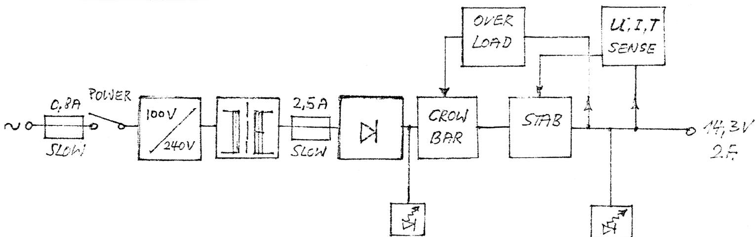
Two light diodes signal the mains and output voltage. Parallel connection of output with external voltage plug by two banana plugs. The position of the switch indicates when the machine is in operation.
