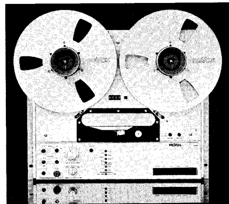
Adjustable on the front panel: treble equalization and 25 Hz-filter circuits.
