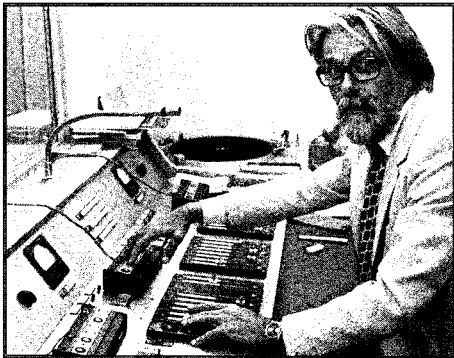
Two veterans of broadcasting: Mr Grossenbacher working at the STUDER vacuum-tube mixing console.
