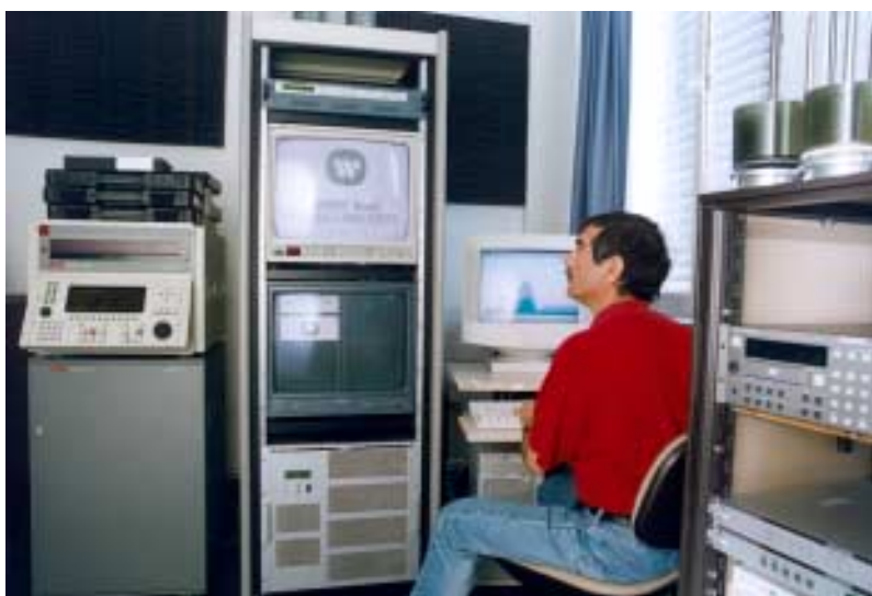
Fig. 2: BTS D1, STUDER DVD 320 Videoencoder Barco Moni- tor, STUDER DVD 310 Audio- encoder, STUDER DVD 315 Audiodecoder, (STUDER D780 DAT Recorder)
