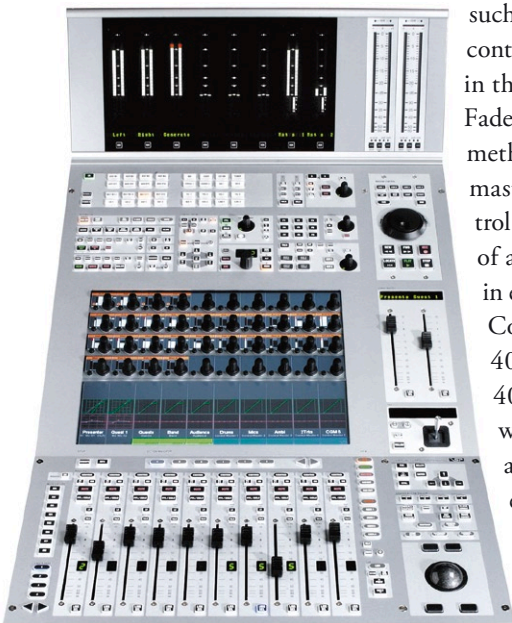
Vista 8 Control Bay
