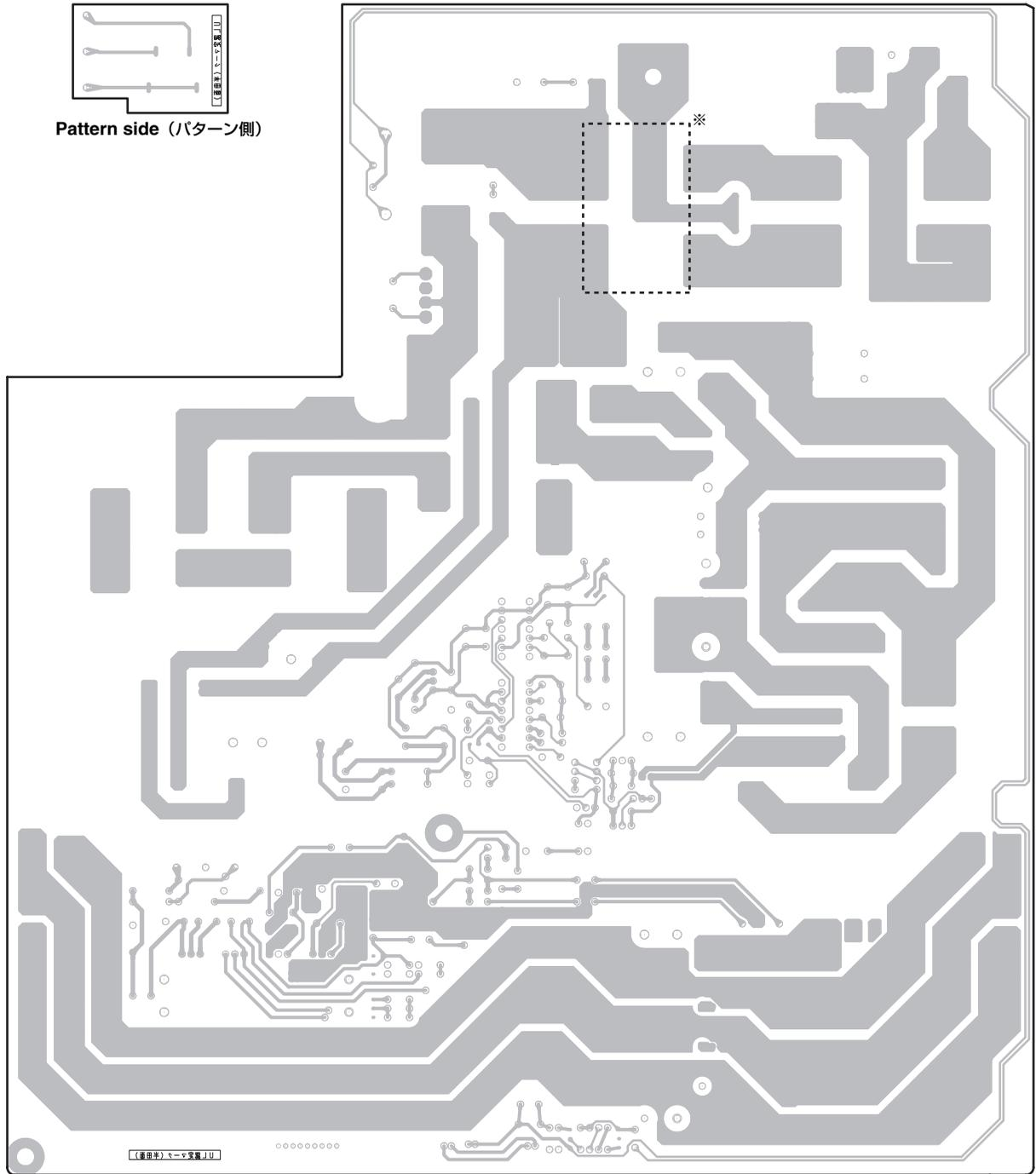
※ The capacitors [C158] and [C159] are attached in the dotted area shown above (U, V, T models).
