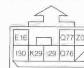
614 : Floor wire No. 1 (To back door wire No. 1 [845])
