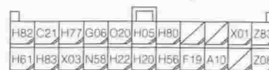
3B2 : Cowl wire LH (To meter 22P)
