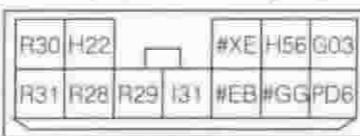
611 : Floor wire No. 1 (To cowl wire RH [3L9])
