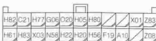
3B2 : Cowl wire LH (To meter 22P)
