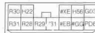
611 : Floor wire No. 1 (To cowl wire RH [3L9])
