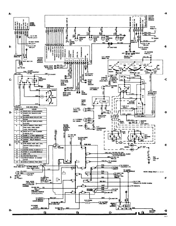
WIRING DIAGRAMS Fig. 5: Instrument Panel (p. 5) 1985 Jeep Cherokee
