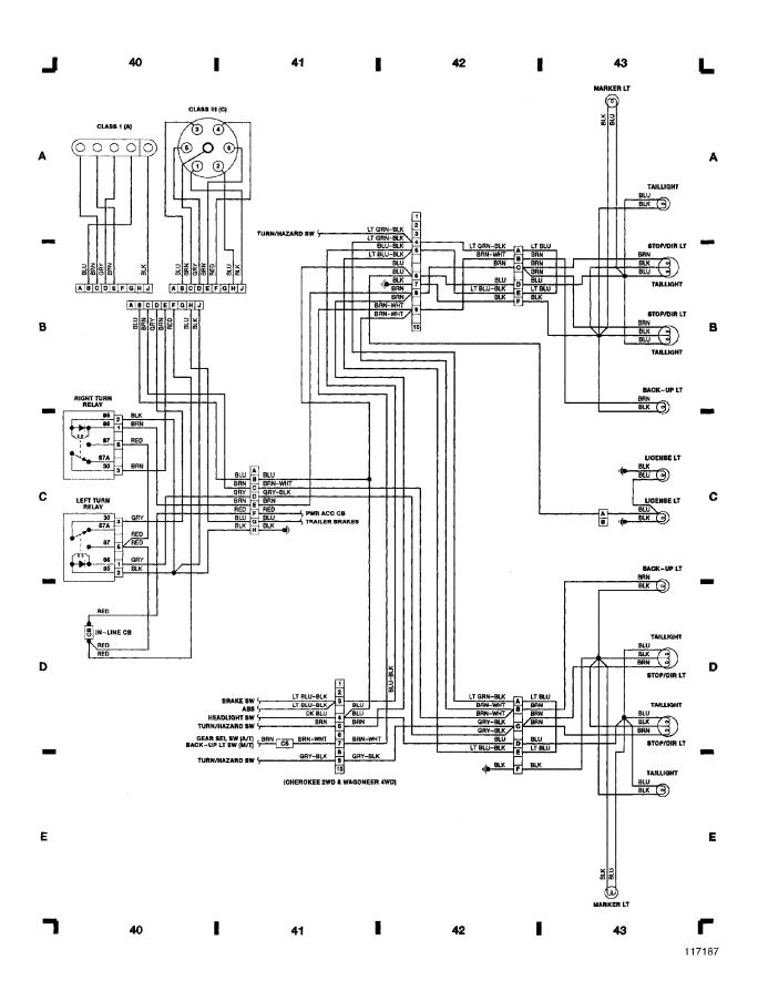
Fig. 12: Towing Package, Taillights (4WD Cherokee) (p. 12)
