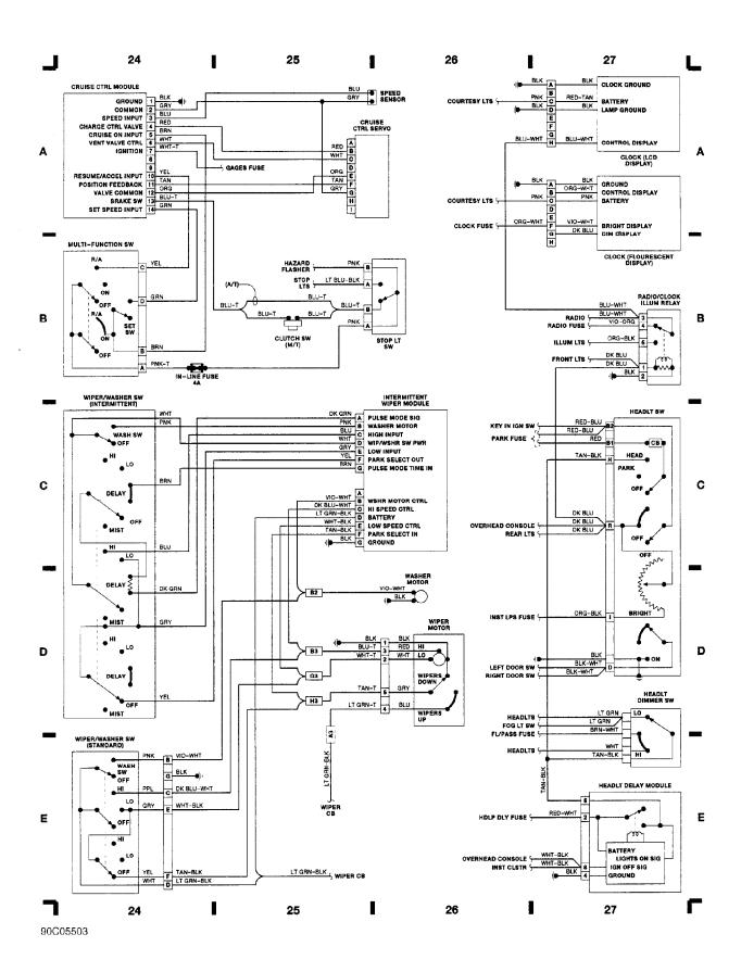
WIRING DIAGRAMS Fig. 8: Instrument Cluster (Standard, Gages, High Line) (p. 8) 1990 Jeep Cherokee
