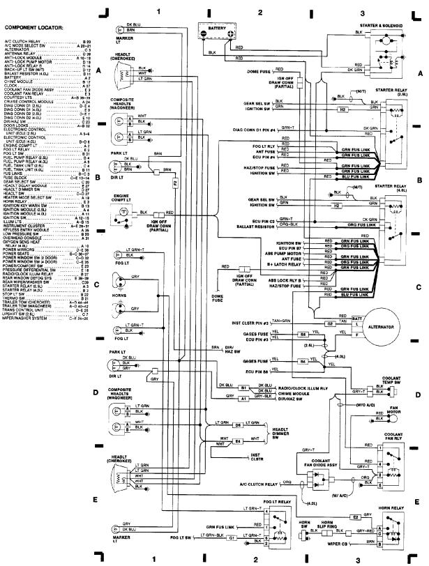
WIRING DIAGRAMS Fig. 2: Electronic Control Unit (ECU) (2.5L) (p. 2) 1990 Jeep Cherokee
