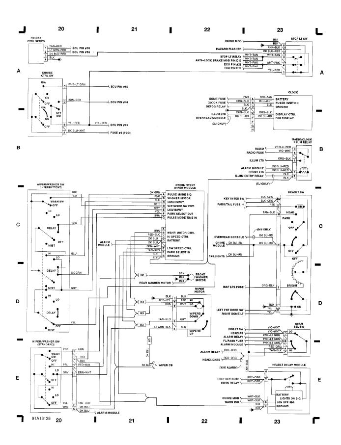
WIRING DIAGRAMS Fig. 7: Alarm Module, Instr Cluster, Warning Indicators (Grids 24-27) (p. 7) 1991 Jeep Cherokee
