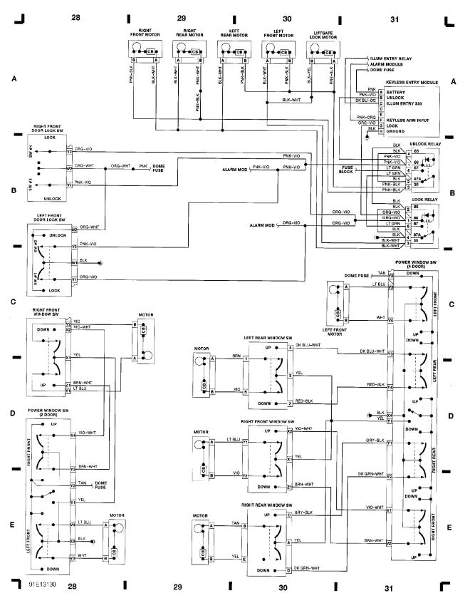
WIRING DIAGRAMS Fig. 9: Passenger Compartment (Grids 32-35) (p. 9) 1991 Jeep Cherokee
