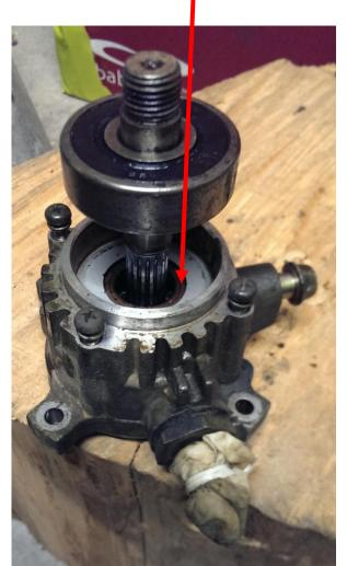
I removed the shaft to check the bearing as well. Because the bearing is in excellent conditions, I haven't replaced it, thus I don't know the size, but if it is wobbling and you have to replace it, just measure it with a caliber.
