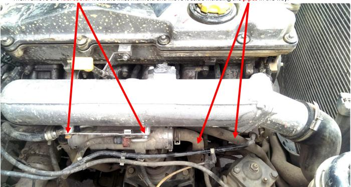
Before removing the belt, I suggest you measure it first, to be 100% sure of which belt you have to buy (I read too many posts of people buying the wrong belt). For the AU version with air conditioning unit it is not a Land Rover belt. It has different length. So I measured it with a wire along the whole path of the belt.
