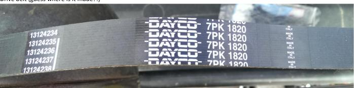
Now you have to remove the drive belt. To do so, use a 15mm spanner to disengage the **drive belt tensioner**, and remove
