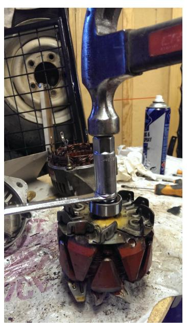
Position the bearing, then place a spanner (the round side over the bearing) sitting on the inner ring of the bearing (I can't remember the spanner size, but be careful that the spanner ring sits only on the bearing inner ring), and use a pipe (I used a hollow socket extension) to push the bearing against the base. Be careful to use a long enough hollow pipe otherwise you will damage the copper contacts.
