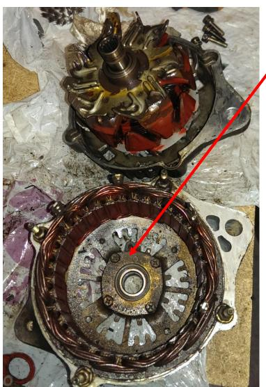
Remove the bearing cover plate,
