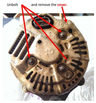
Remove the bolts (screw them back in after removing all parts) to remove the **regulator**, the **brushes**, and the **rectifier**
