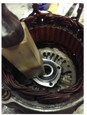
Insert the other bearing in the alternator case. I used a wood stick because it is not possible to reach it with the hammer, and using a wood stick rather than a metal stick will avoid to damage the bearing. Hit the bearing only on the edge.
