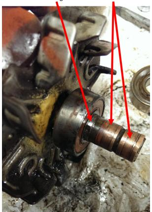
Use an extractor to remove the bearing (OD=35mm, ID=15mm, th=13mm)
