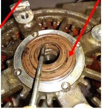
Remove the bearing (OD=40mm, ID=17mm, th=12mm) hitting with a hammer on a 22mm socket seated on the bearing.
