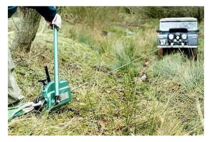
There are three sizes of Brano hand winches available. The smaller size is quite suitable for use with all smaller sized 4x4s, including SWB Land Rovers, Ninetys, Range Rovers and Discoverys. Though I recommend you carry a Superwinch Swingaway snatch block with this size.
