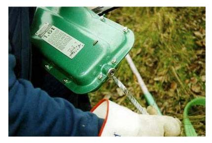
Inserting the tapered end of the wire rope (see picture below).
