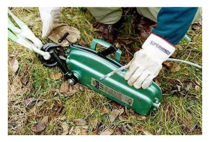
Make sure your wire rope is always in good condition, not only for safety's sake, but also damaged wire rope will not 'run through' the 'jaws' of the Brano. To ensure that you get no kinks in the wire rope, when taking the rope off the carrier, drop the hook end to the ground and walk forward unrolling the rope. Simply dragging the wire rope off the side of the carrier will cause all sorts of problems of untwisting of the lay and kinking. You have been warned!
