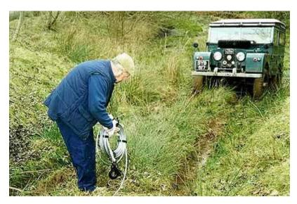
With the Brano you can pull at any angle you like, on any secure point on an end or side of the vehicle. On a drum winch you must of course only pull in the cable square to the drum to avoid problems.
