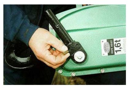
The shear pin is installed in this position (see picture).
