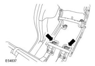
**4.** Check that the rear seat frame front fixings are secure and that the seat frames show no signs of movement. Front seat frame fixings - Every 2 years or 30,000 miles (48,000 km)
