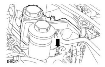
WARNING: Since injury such as scalding could be caused by escaping steam or coolant, do not remove the filler cap from the coolant expansion tank whilst the system is hot.
