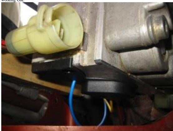
Rather than fit the new shuttle valve switch module, then find that the problem was the internal connections in the ABS unit, I decided to perform the modification to bypass the possibly faulty internal connections.
