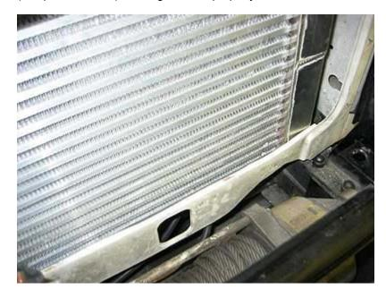
Here you can see the front panel in place with the removed edge. Make sure it is not sharp because it might otherwise damage the intercooler core. The front panel on my vehicle is a bit bent and butchered but it if you've got a straight one it will look better (see picture above).
