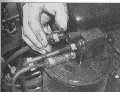
54.3 Disconnect the wiring plug from the purge valve
