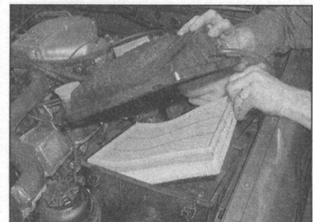
9.14 . . . then lift up the lid and remove the filter element
