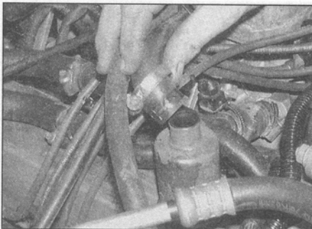
10.9 Disconnect the hose from the crankcase filter
