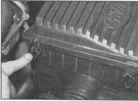
10.15 Releasing an air cleaner lid securing clip - 300 TDi engine
