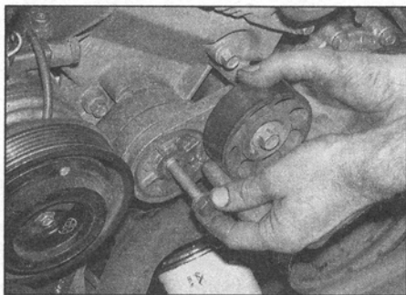
8.5a Remove the drivebelt tensioner mounting bolt . . .
