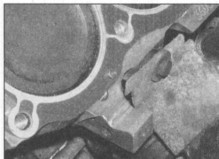
8.27b . . . and locate it over the dowels
