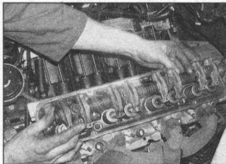
6.31 Offer the rocker gear into position, aligning the pushrods and rockers
