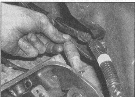
8.7b . . . and where applicable, unclip the lambda sensor wiring connector
