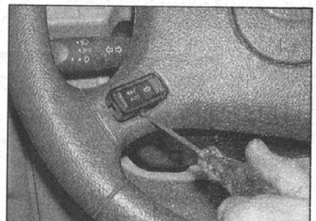
13.15 Prise out the cruise control switches from the steering wheel . . .
