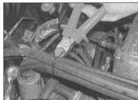
3.3 This cable-tie had to be cut to release the cable
