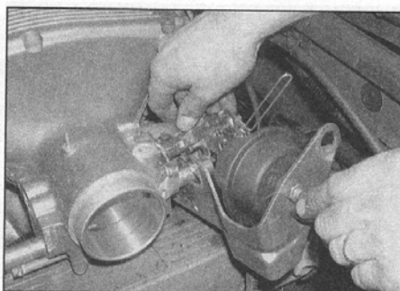
6.56f Remove the throttle linkage assembly, and place to one side
