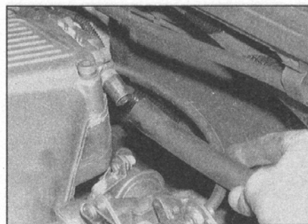
6.68a Disconnect the air by-pass valve hose for access ...
