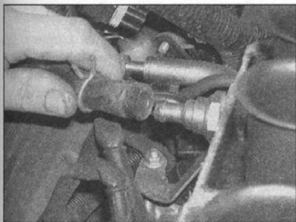
6.61b ... the brake servo vacuum hose ...
