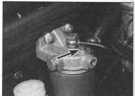
5.3 Fuel filter head bleed screw (arrowed)
