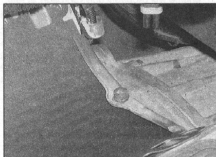
9.22 Gasket clamp in position
