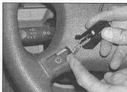
22.16 ... and disconnect the wiring
