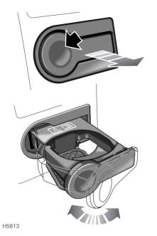
Press to open (solid arrow). When the holder is open, the leading edge can be pivoted out (as lower illustration) to adjust the aperture to suit the size of the cup. Push the cup holder in to close.
