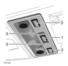
Front interior light and map lights illustrated The interior light illuminates automatically whenever the vehicle is unlocked, when the starter switch is turned off (provided the sidelamps have been on in the last 30 seconds), or when a door or taildoor is opened. The light remains illuminated for 20 seconds after the doors and taildoor are closed, or until the starter switch is turned on.
