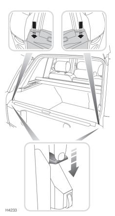
With the upper taildoor open, push down on the two hidden catches (see upper insets), either side of the taildoor. The catches can be operated either one at a time or simultaneously.
