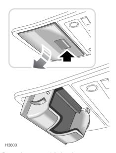
Press where arrowed (in inset) to open.
