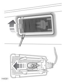
Insert a small flat-bladed screwdriver under the lens and carefully prise the lens from the light unit. Pull the bulb to remove.
