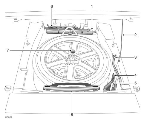
The wheel change tool kit is stowed in the spare wheel well, under an access hatch in the rear loadspace area.
