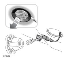
Insert a small flat-bladed screwdriver under the side of the light unit and carefully prise the unit out of the footwell.
