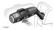
Push the lever away from the steering wheel to change headlamps to high beam (BLUE warning light illuminates). Pull the lever back towards the steering wheel to change back to normal beam headlamps.
