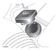
With the engine warm (to assist oil drainage) and the vehicle parked on firm, level ground, remove the filler cap and position a container of suitable size (at least 10 US quarts or 10 litres) under the drain plug, in the bottom of the sump.
