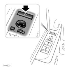
Access height can be selected when in any ride height, by either pushing the ride height selector down when in standard or motorway ride height, or by pressing the access height switch on the driver's door switch panel (arrowed above).
