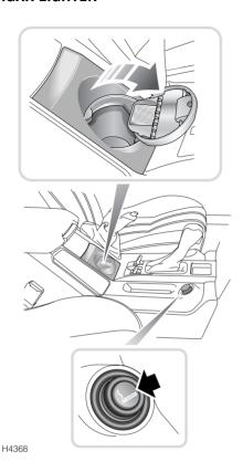
With the starter switch turned on, press the lighter in (lower arrow) to heat up. When it has reached the correct temperature it will partially eject and can then be withdrawn for use.
