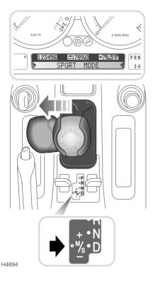
In Sport mode, full automatic progression through the gear ratios is retained. By selecting Sport mode, however, the power transmitted to the road wheels is increased by making lower gears more available. This results in improved mid-range performance, as the vehicle stays in the lower gears for longer. Sport mode also makes the lower gears more available for 'kick-down' operation.
