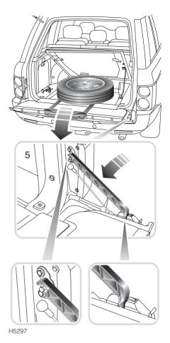
5. Once the wheel has been lifted onto the taildoor, attach the hinge-stop, to prevent the taildoor from lifting. Remove the spare wheel from the load space area.
