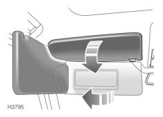
Pivot the sun visor downward to reduce sun glare through the front windshield. If required, the visor can then be pivoted towards the side window to reduce sun glare from that side of the vehicle.
