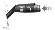
This feature can also be activated by pressing the button on the end of the lever.
