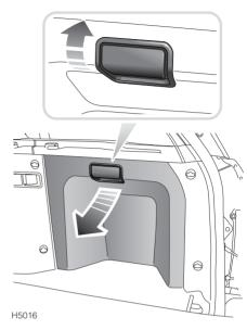
The access hatch is located on the right hand side of the rear loadspace and provides access to the warning triangle\*, the rear loadspace fuse box and the emergency fuel filler flap release.
