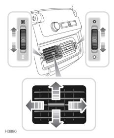
The left hand control operates the blower; rotate the thumbwheel upwards to increase the blower speed. The right hand control adjusts the temperature; rotate the thumbwheel upwards (red indicator) for warmer air, downwards (blue indicator) for cooler air.
