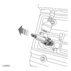
**12.** Clean the area around each spark plug and, using a suitable spark plug wrench, remove 8 spark plugs.
