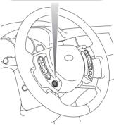
Press to activate the steering wheel heating elements. The heating elements are thermostatically controlled and operate intermittently (when switched on) to maintain a comfortable temperature. Press the switch again to manually deactivate the heater.
