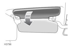
A secondary sun visor is located behind the main visor and can be used as required.
