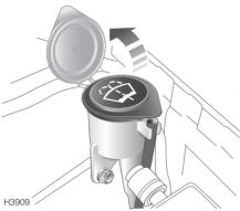
The windshield washer reservoir supplies both front shield and rear screen washer jets and headlamp washer jets \*.
