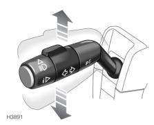
Move the lever DOWN to indicate a LEFT turn, and UP to indicate a RIGHT turn (the appropriate GREEN warning light on the instrument panel will flash in time with the direction indicators). Hold the lever part-way up or down against spring pressure to indicate a lane change.
