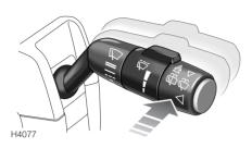
Push the lever forward to the first position, then forward again and hold against spring pressure for the required duration of window washing. The wiper operates automatically during washing and continues for a further 3 wipes after the switch is released.
