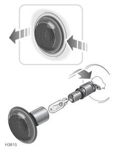
Push the lens firmly towards the front of the vehicle and withdraw the lamp unit from the fender. Twist to release the bulb holder from the lens unit, then pull the bulb from its socket.
