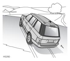
Approach at right angles so that both front wheels cross the ridge together - an angled approach could cause stability to be lost through diagonally opposite wheels lifting from the ground at the same time.
