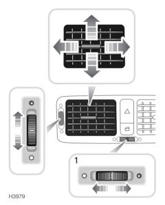
When the air conditioning air distribution control is set to either 'Auto' or 'Face and Foot' outlet, the temperature of the air emitted through the foot/face level vents can be finely adjusted to differentiate between foot and face temperature. Rotate the thumbwheel (1), towards the left (red indicator) for warm air and to the right (blue indicator) for cooler air.
