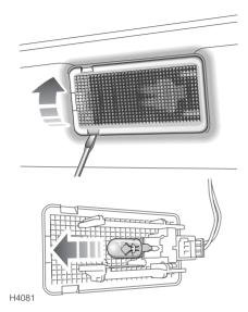
With the relevant door open, insert a small flat-bladed screwdriver under the forward edge of the lens. to lever the light unit out of the door. Pull the bulb out to remove.
