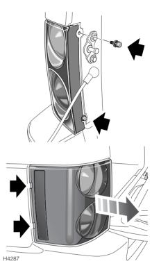
From outside the vehicle and with the taildoor fully open, remove the two retaining screws (as shown). From the side of the vehicle, use a suitable tool to carefully lever the unit away from the vehicle and rearwards, to access the side marker bulb holder.
