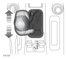
CommandShift gear selection can be used as an alternative to fully automatic transmission and is particularly effective when rapid acceleration or engine braking into corner and descents are required.
