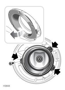
To access the bulb; using a suitable tool, lever the fog lamp surround panel out of the front bumper. Remove the three securing screws to release the lamp unit. Ease the unit out of the front bumper.
