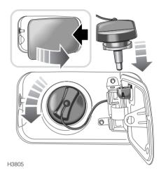
The fuel filler is located in the rear right-hand fender. With the vehicle fully unlocked (all doors and taildoor), press the right side of the fuel filler flap to open (shown in inset).
