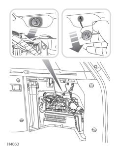
If the vehicle battery has been disconnected or has discharged, the fuel filler flap can be opened manually. Open the rear loadspace access hatch (see **REAR LOADSPACE ACCESS HATCH**, **120**). Pull the green release handle (as illustrated in the insets) to open the filler flap.
