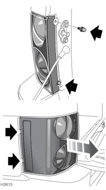
From outside the vehicle and with the taildoor fully open, remove the two retaining screws (as shown). From the side of the vehicle, use a suitable tool to carefully lever the unit away from the vehicle and rearwards, to release the lamp unit from the vehicle.
