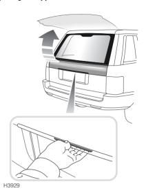
With all doors unlocked, press the switch on the bottom edge of the upper taildoor and lift to open.
