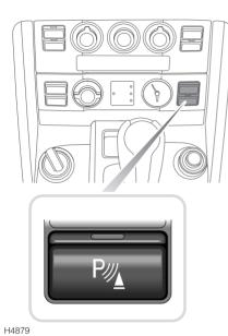
PDC can also be manually selected by pressing the switch (illustrated) on the centre front facia (the indicator light in the switch illuminates and a short tone sounds as confirmation). A second press of the switch deactivates the PDC system. If PDC has been manually switched off by pressing the switch, it will not activate automatically until either the switch has been pressed again, or the starter switch has been turned off and on again.
