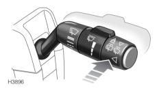
Push the lever forward to the first position to operate, the wiper operates intermittently until switched off.
