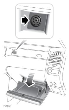
Press the release button (arrowed in inset) to open.
