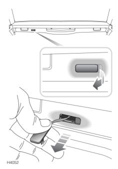
If the battery has been disconnected or has discharged, the taildoor can be opened manually as follows:
