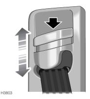
The height of the seat belt upper anchorage can be adjusted for comfort AND safety on both front seats and also the two outer rear seats. Press down (solid arrow) to release the catch, then lift or push down to adjust the height of the anchorage. For safety, the seat belt should always be worn with the webbing crossing the shoulder MIDWAY BETWEEN THE NECK AND THE EDGE OF THE SHOULDER.
