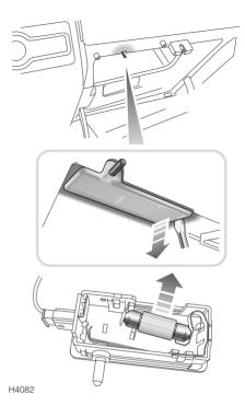
Insert a small flat-bladed screwdriver into the indent (see inset) on the side of the light unit, and carefully prise the unit from the glovebox panel. Remove the bulb from its clips.
