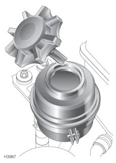
Wipe the filler cap clean to prevent dirt from entering the reservoir. Remove the filler cap and, using a lint-free cloth, wipe the dipstick clean. Refit the filler cap fully and remove it again to check the fluid level. Add fluid to the reservoir until the level is between the upper mark and the bottom of the dipstick. **DO NOT fill above the upper mark on the dipstick.**
