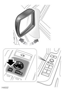
Press the mirror-fold button (arrowed in inset) once to fold the mirrors into the side windows. Press again to return the mirrors to the driving position.
