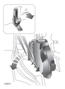
Pull the release lever (see inset) rearwards, then push the seat assembly back onto the floor - the floor catches should latch with the base of the seat. Then raise the backrest
