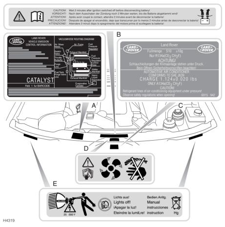
Various labels are fixed inside the engine compartment, the number, position and content of which may vary from model to model. The following illustration locates labels of specific importance and is included for guidance only.
