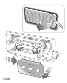
Insert a small flat-bladed screwdriver into the indent on the side of the lens and carefully prise the lens from the light unit (see inset).
