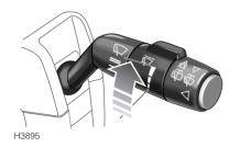
With the lever in position '1', rotate the switch clockwise to increase and counter-clockwise to decrease the frequency of the intermittent wipe.
