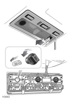
Insert a small flat-bladed screwdriver into the indent on the side of the lens (as illustrated) and prise the lens from the light unit. Twist the relevant bulb holder counter-clockwise and withdraw from the light unit, then pull the bulb out to remove.
