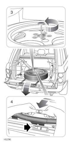
4. Attach the spare wheel lifting strap handle to the top of the lower taildoor (as inset 4), ensuring that the two lugs engage fully with the corresponding apertures in the top of the taildoor. Once the handle is correctly located, the taildoor is automatically released. Lower the taildoor; the wheel lifting strap automatically raises the wheel out of the spare wheel well and onto the lower taildoor, therefore improving ease of removal.
