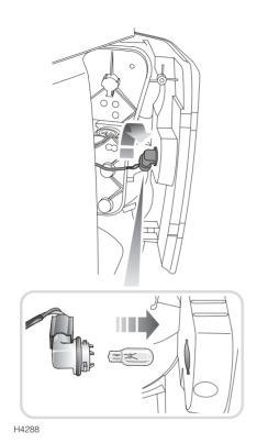
Twist the bulb holder to release it from the lamp unit (as arrowed in illustration), then pull the bulb to remove (see inset).
