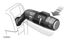
Pull the lever towards the steering wheel (for at least 0.5 seconds). The windshield wipers will operate in conjunction with the washers for as long as the lever is held in this position, the wipers continuing for a further 3 wipes after the lever is released.
