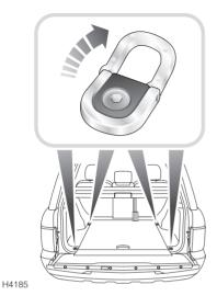
Four fixing points are provided in the rear loadspace floor, to assist in safely securing large items of luggage. Land Rover provide a range of approved luggage retention accessories.
