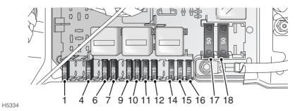
The fuse box is situated on the right hand side of the loadspace behind the rear loadspace access hatch. Pull the handle to open the panel - see **REAR LOADSPACE ACCESS HATCH**, 120.
