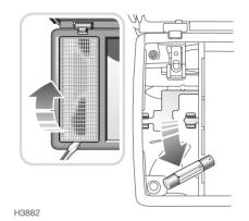
With the vanity mirror cover open, use a small flat-bladed screwdriver to lever the relevant lens from the mirror/light unit. Pull out bulb to remove.
