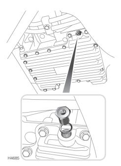
Remove the drain plug and copper washer and allow the engine oil to drain into the container.
