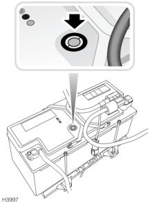
**Note:** When checking the battery condition indicator, if necessary, clean the battery top to ensure a clear view.
