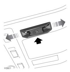
The electric sunroof can be operated when the starter switch is at position 'I' or 'II', and for up to 16 minutes after the starter switch is turned off (provided a front door is not opened).
