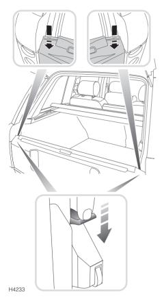
With the upper taildoor open, push down on the two hidden catches (see upper insets), either side of the taildoor. The catches can be operated either one at a time, or simultaneously.
