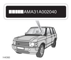
In addition, the Federal VIN plate is mounted to the vehicle body so that it is visible through the lowest part of the left side of the windshield.
