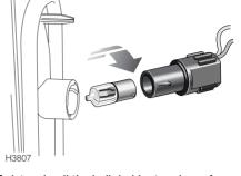
Twist and pull the bulb holder to release from the rear of the lamp unit, then pull the bulb to remove.
