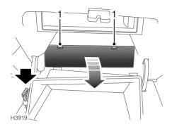
The passenger compartment fuse box is fitted behind the glovebox; to access the fuses, open the glovebox, then press down on the catches (1) whilst pulling the cover rearwards. The solid arrow in the illustration indicates the location of the fuse removal tool.
