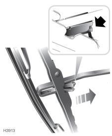
Lift the wiper arm away from the rear screen and pivot the blade assembly away from the arm. Press the tab (arrowed in inset), to release the blade assembly and slide the assembly off the end of the wiper arm. Carefully replace the arm to its stowed position.
