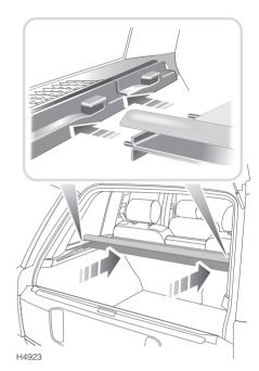
Place the loadspace cover in position, ensuring that the two locating pins on each side rest on the slides just rearwards of the sockets.
