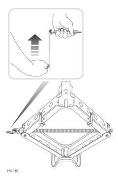
Position the jack under the relevant jacking point, attach the jack cranking handle to the jack. Turn the jack handle clockwise to raise the jack cradle until it engages with the jacking point. Ensure that the base of the jack is in full contact with the road surface.
