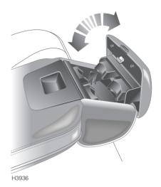
With the armrest folded down, depress the release catch and fold out the double cup holder (mounted in the back of the centre seat headrest).
