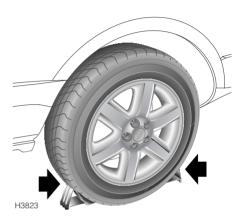
If possible, position the vehicle on level ground, chocking both sides of the wheel diagonally opposite the one to be removed.
