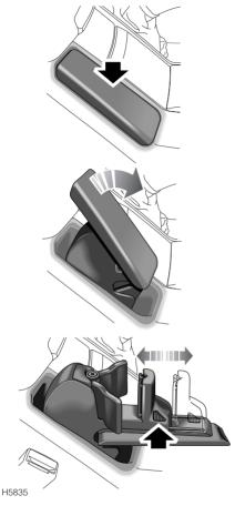
Push the middle of the cover to open (upper solid arrow). Push the cover forwards to open the cup holder. Press the catch (lower solid arrow) and slide the cup holder clamp to adjust the aperture to suit the size of the cup.
