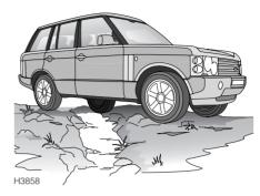
Cross ditches at an angle so that three wheels always maintain contact with the ground. If a ditch is approached head on, both front wheels will drop into the ditch together, possibly resulting in the chassis and front bumper being trapped on opposite sides of the ditch. If the severity of terrain makes this inevitable, selecting 'Off-road' height with the EAS to increase clearance between the ground and the bottom of the vehicle may help.
