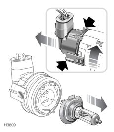
Depress the two catches (solid arrows in upper inset), then twist and pull to remove the bulb holder from the lens assembly. Pull the bulb from the holder to remove.
