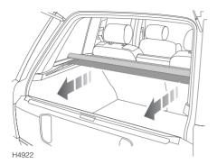
With the cover folded, pull the whole assembly rearwards to disconnect the locating pins and withdraw the loadspace cover carefully from the vehicle.
