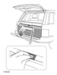
With the upper taildoor open, press the release switch on the top of the lower taildoor (see inset), then lower the taildoor.
