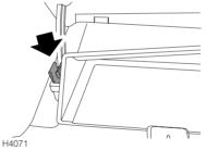
The fuse removal tweezers are located in the glovebox (arrowed in illustration). Press the tweezers onto the head of the suspect fuse (as shown) and pull to remove. A break in the wire inside the fuse indicates that the fuse has 'blown' and must be replaced.
