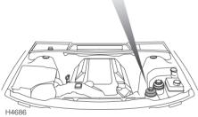
The engine oil filter is located at the front of the engine compartment.
