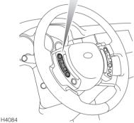
Cruise control enables the driver to maintain a constant road speed without using the accelerator pedal. This is particularly useful for motorway cruising or for any journey where a constant speed can be maintained for a lengthy period.
