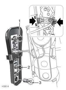
Press the two tabs (arrowed in inset) together, to release the lamp unit from the lens assembly. Twist and pull the appropriate bulb to release.
