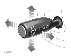
The steering wheel position can be adjusted in four directions, corresponding with the movement of the adjustment lever, to suit your driving position.
