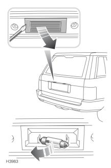
With the upper taildoor open and using a suitable tool, lever the lens from the taildoor (see inset). Pull the bulb to remove.
