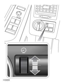
Rotate the control upwards to increase, or down to decrease, the intensity of the instrument panel illumination.
