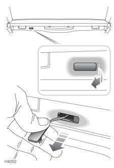
If the battery has been disconnected or has discharged, the taildoor can be opened manually as follows:
