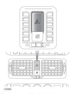
Press to operate; all the direction indicator lamps (including those fitted to a trailer) will flash together. Use ONLY in an emergency to warn other road users when your stationary vehicle is causing an obstruction, or is in a hazardous situation. Remember to switch off before moving away.
