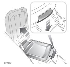
Press down on the catch and lift up the main lid of the cubby box to access the trinket tray.
