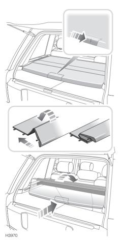
Push firmly downwards and forwards on the centre of the rear edge of the cover (where arrowed in the upper inset), then lift and fold forwards.
