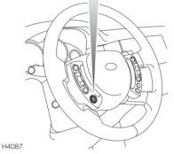
Press to turn air recirculation on or off. The indicator light in the main recirculation control will illuminate when air recirculation is active.
