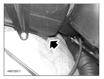
Confirm satisfactory operation of the valve by pouring a small quantity of water through the air intake on top of the wing, ensuring that the water drains through the valve unaided.
