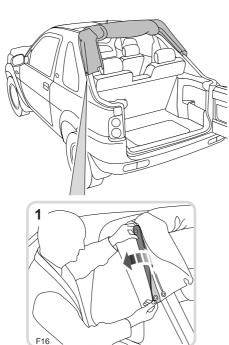
Unfasten the side cover velcro and stud fasteners.
