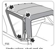
Undo velcro, stud and zip fasteners.
