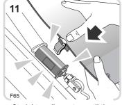
Straighten elbow stay until the locking collar 'snaps' up. Attach corner post clips to locking collar.
