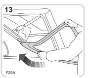
Slide the side screen up the retaining channel, using a series of short pushes, positioning the hands where shown.
