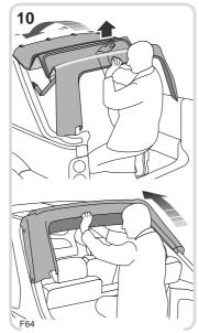
While pushing upwards on the centre roof bow, fold softback forwards.
