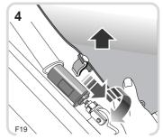
Detach corner post clips. Push and twist to release elbow stay locking collar.
