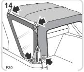
Attach zip, stud and velcro fasteners.
