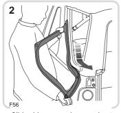
Slide side screen down and out of the retaining channel.
