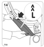
Feed appropriate side cover ('L' or 'R') into the retaining channel in the direction of the chevrons.
