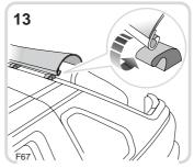
Hook leading edge of tonneau cover over the four hooks.
