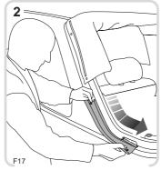
Slide the cover out of the retaining channel.
