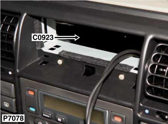
Description: Head Unit-Audio System Location: Behind radio
