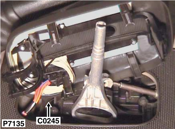
Description: Lamp-Automatic gearbox selector indicator Location: Beneath centre console
