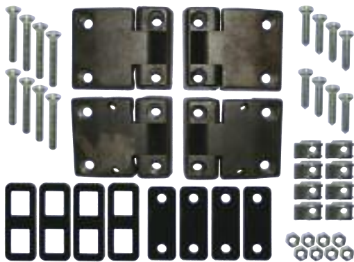
DA1069 Front door hinge kit for Series 3 and 90 & 110 Defender
