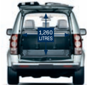
Maximum loadspace behind row 2 – seats up
