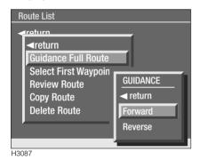
If you want to reverse the direction of the route you are following, highlight and select 'Guidance Full Route', then highlight and select 'Reverse'. The navigation computer returns to the route guidance screen while calculating the new route and new audio instructions are given.
