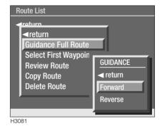
The navigation computer requests the desired route direction (a route can be followed in the opposite direction to which it was programmed), highlight and select the chosen direction. The navigation computer returns to the route guidance screen and audio instructions are given (see 'Route guidance').
