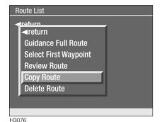
Rename the route using the rotary select control to highlight and select the letters from the typewriter menu, then highlight and select 'enter'. The 'Review Route' screen is displayed - edit the required waypoints as described in 'Waypoints' later in this section, before storing in the route list.
