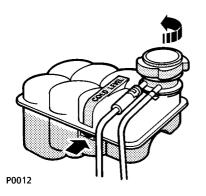
Top-up to the arrowhead (next to the seam) on the side of the tank with a 50% mixture of anti-freeze and water. Ensure the cap is tightened fully after top-up is completed.
