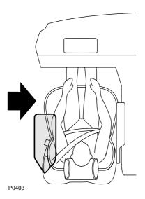
Airbag inflation is virtually instantaneous and occurs with considerable force accompanied by a loud noise. The inflated airbag, together with the seat belt restraint system, limit the occupant's movement, thereby reducing the risk of injury to the head and upper torso.
