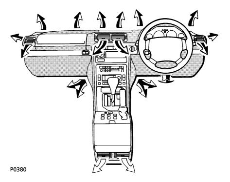
The heating and ventilation system provides fresh or heated air to the vehicle occupants. Outlets are positioned to supply air at both face and foot level and also to the windscreen, as well as to a single lap cooler vent positioned below the steering wheel. The location of the vents is shown in the illustration.
