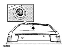
To adjust the rear screen washer jet, insert a long needle-like probe into the jet orifice and lever gently to position the jet so that the spray is directed towards the cross symbol on the screen.
