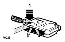
Press to release the key, which can then be used as a conventional key to operate the starter switch, glovebox and door locks
