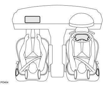
To ensure correct deployment of the airbags, it is essential that obstructions are not allowed to intervene between an airbag and the occupant. The following are examples of the type of obstructions that could either, impede correct operation of the airbags, or jeopardise personal safety in the event of an airbag deployment:
