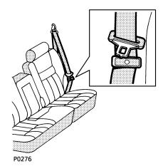
Before folding either part of the rear seat, ensure that the outer rear seat belts are correctly stowed in their belt clips (see illustration). To avoid damaging the centre seat belt, roll the buckle neatly and stow it in the space provided at its anchor point in the centre of the rear seat.
