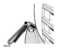
Should any jet become obstructed, insert a needle or a strand of wire into the orifice to clear it.
