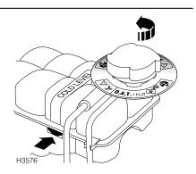
Top-up to the arrowhead (next to the seam) on the side of the tank with a 50% mixture of anti-freeze and water. Ensure the cap is tightened fully after top-up is completed.
