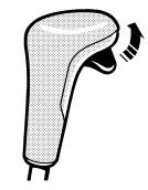
A spring loaded catch built into the handle of the gear selector lever restricts movement of the lever, thereby preventing inadvertent gear selection. The catch has two pressures:
