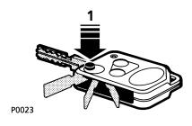
Press to release the key, which can then be used as a conventional key to operate the starter switch, glovebox and door locks.
