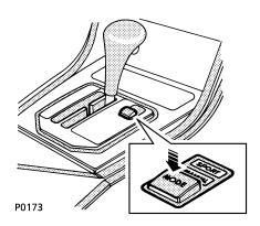
To select 'Sport' mode, press the 'Mode' switch once whilst the gearbox is in High range (the message centre will display 'S' along with the selected gear, eg. 'S3').
