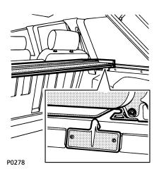
The loadspace cover can be removed by pulling on the rear to disengage it from the side spigots and stored in the forward area of the loadspace; a channel is formed in both of the loadspace side panels immediately behind the rear seats to accommodate the folded loadspace cover.
