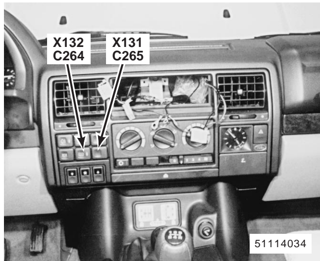
100. centre of fascia X131 Heated Front Screen Switch X132 Heated Rear Screen Switch C264 (5-U) C265 (5-U)
