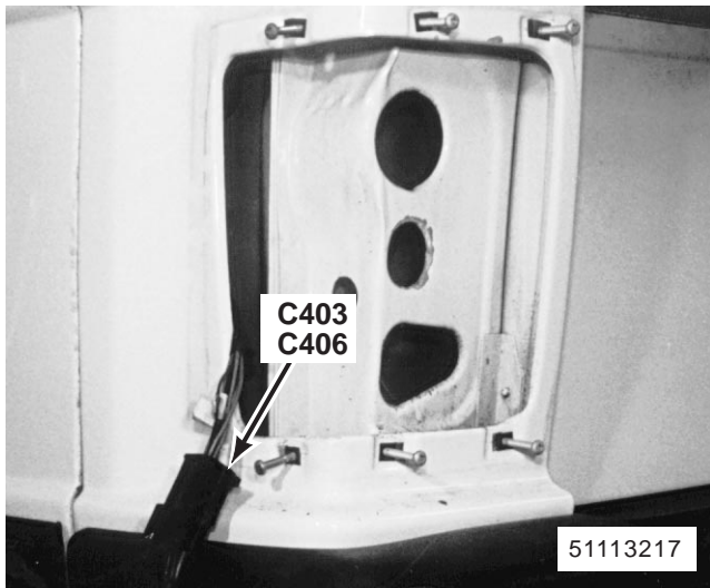
219. LH side of rear bumper (RH similar) C403 (6-B) (Left) C406 (6-B) (Right)
