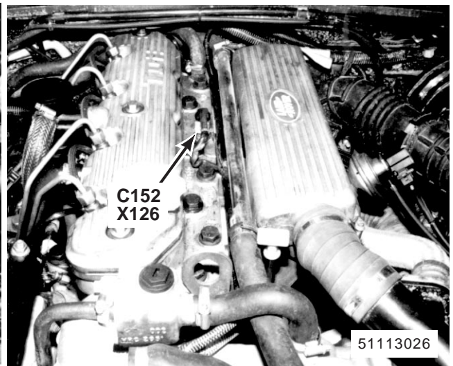
24. top centre front of engine Diesel X126 Engine Coolant Temperature Sensor C152 (2-N)
