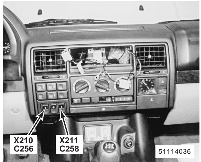
102. centre of fascia X210 Air Suspension Up Switch X211 Air Suspension Down Switch C256 (6-R) C258 (6-G)
