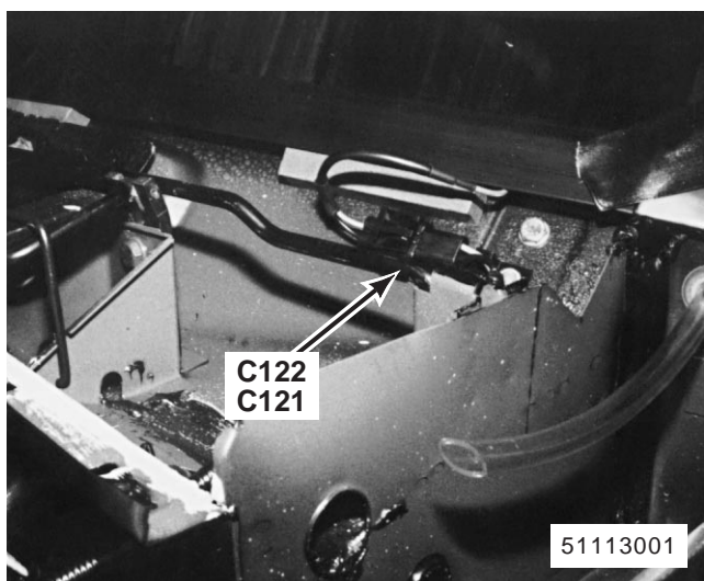
1. lower LH side of windscreen (RH similar) C121 (2-B) (Right) C122 (2-B) (Left)
