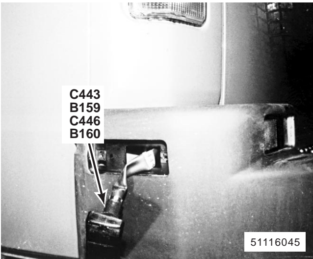
187. LH side of rear bumper (RH similar) B159 Left Rear Side Marker Lamp B160 Right Rear Side Marker Lamp C443 (2-B) C446 (2-B)
