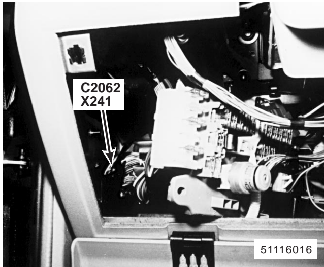
93. behind LH side of fascia left of steering column X241 Saudi Junction Connector C2062 (1-B)
