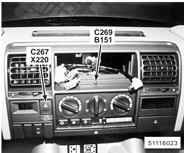
115. centre of fascia X220 Hazard Switch B151 Theft Alarm LED C267 (10-B) C269 (2- )
