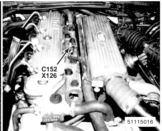
26. top centre front of engine (300Tdi without EDC)
