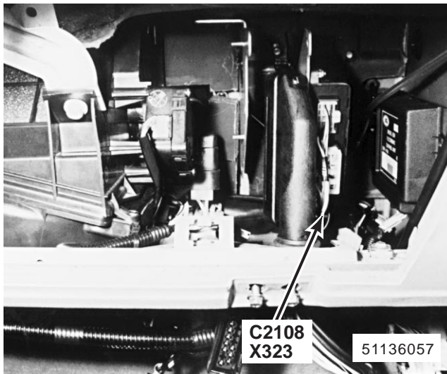
185. behind RH side of fascia (Early Production) X323 Data Link Connector (Theft Alarm) (Early Production) C2108 (4-B) (Early Production)
