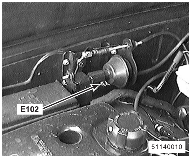
53. RH rear of engine compartment (300Tdi) E102
