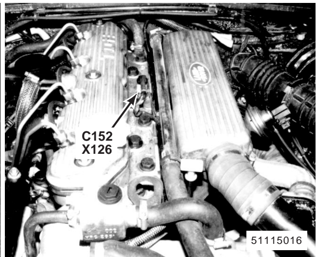
26. top centre front of engine (300Tdi without EDC) X126 Engine Coolant Temperature Sensor C152 (2-N)
