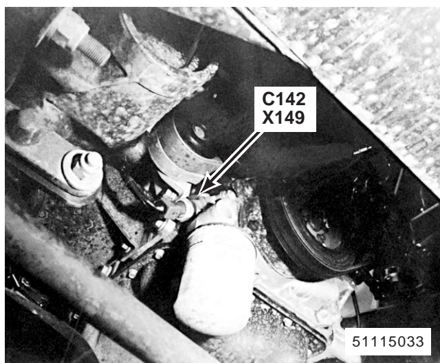
47. lower RH side of engine (MFI-T16) X149 Oil Pressure Switch C142 (2-N)
