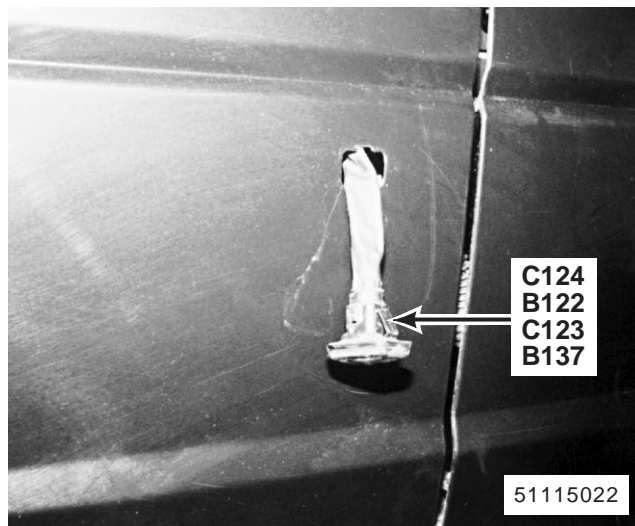
32. LH front side of vehicle (RH similar) B122 Left Repeater Lamp B137 Right Repeater Lamp C123 (2-B) (Right) C124 (2-B) (Left)
