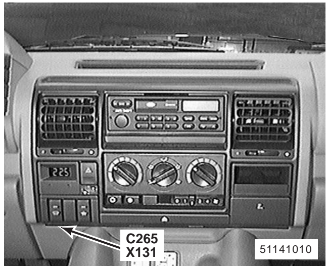
268. centre of fascia X131 Heated Front Screen Switch C265 (5-B)
