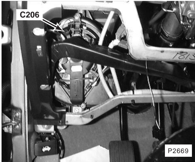
73. behind driver's side of fascia (lower dash panel removed) C206 (1-B)
