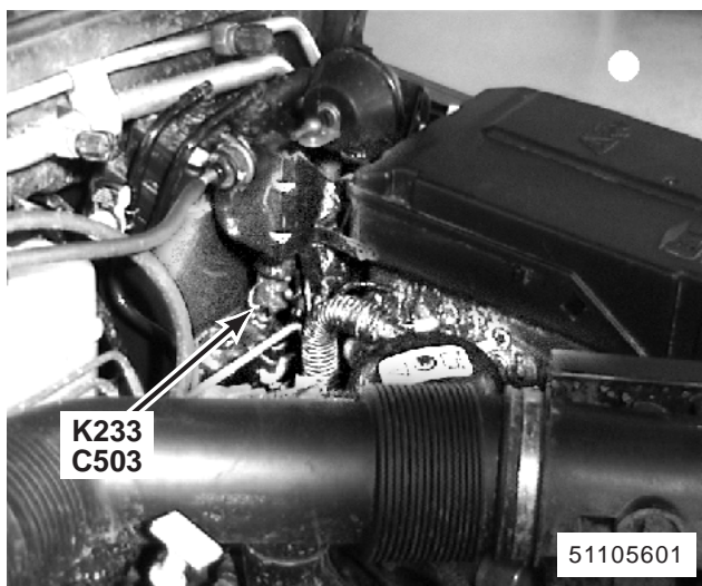
280. LH rear corner of engine compartment K233 Evaporative Emission Canister Vent Seal Valve C503 (2-R)
