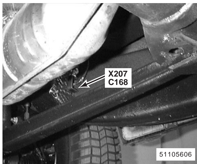
46. beneath RH side of vehicle X207 Right Front Height Sensor C168 (3-B)
