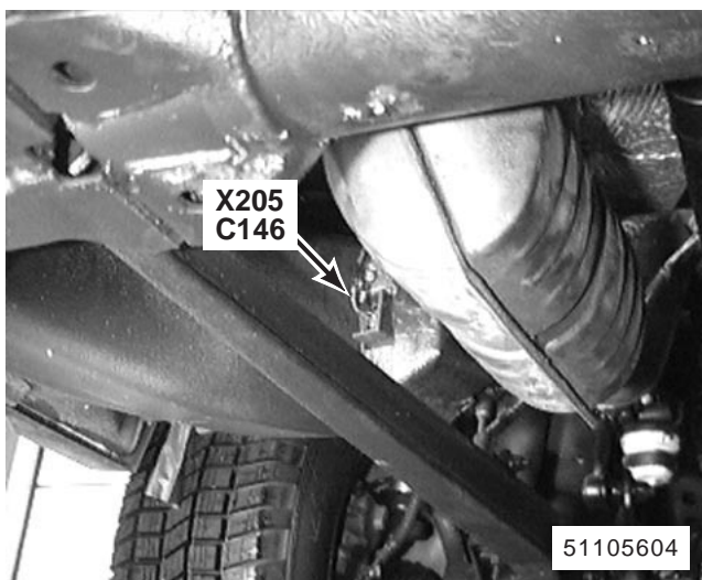
47. beneath RH side of vehicle X205 Left Front Height Sensor C146 (3-B)
