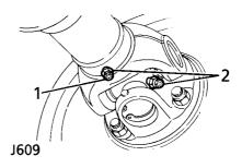
Clean all the grease nipples on the front and rear propshaft universal joints (1). Charge a low pressure hand grease gun with the recommended grade of grease (see 'General data') and apply to the grease nipples (2).
