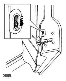
**Child-proof locks** - 110 Station Wagons Move the locking levers to the 'ON' position (as illustration) to engage.
