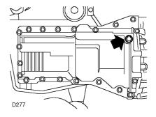
• Remove the drain plug and discard the sealing washer. Allow the oil to drain completely.
