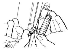
Open the sunroof fully and push the catch (1) rearwards to disengage the hand wheel mechanism.
