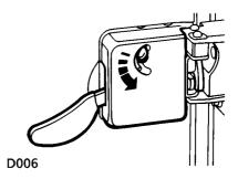
**Rear door** - (if fitted) From outside, use the key to lock and unlock. From inside and with the door closed, push the locking button up to lock and down to unlock (as illustration).
