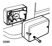
**Reverse and rear fog guard lights** Remove the retaining screws and withdraw the lens, then push and twist to release the bulb.
