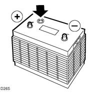
The battery is designed to be maintenance free, so topping-up is not possible. On the top of the battery there is a battery condition indicator (arrowed in illustration). Examine the indicator periodically to check the battery's condition. When the indicator shows:
