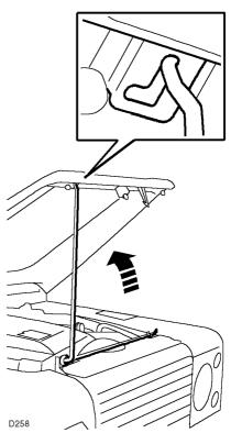
Unclip the stay from the bonnet locking platform and fit the stay in the corresponding slot in the underside of the bonnet.
